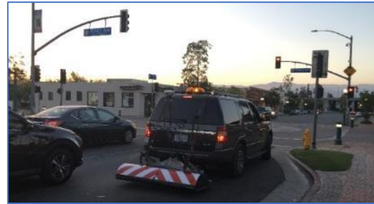
Figure 92 Typical environment in which GPR-Array data is gathered
