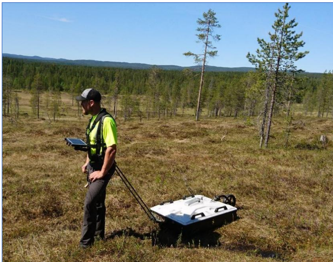
Figure 9 Practical use of the waist belt, pulling rods, handle, and pad-harness.
