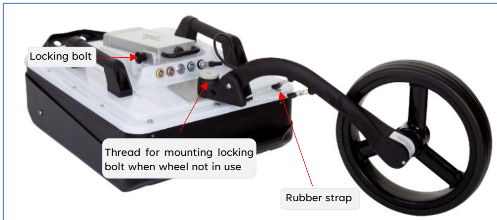
Figure 8 Single measuring wheel attached with the GPR system.
