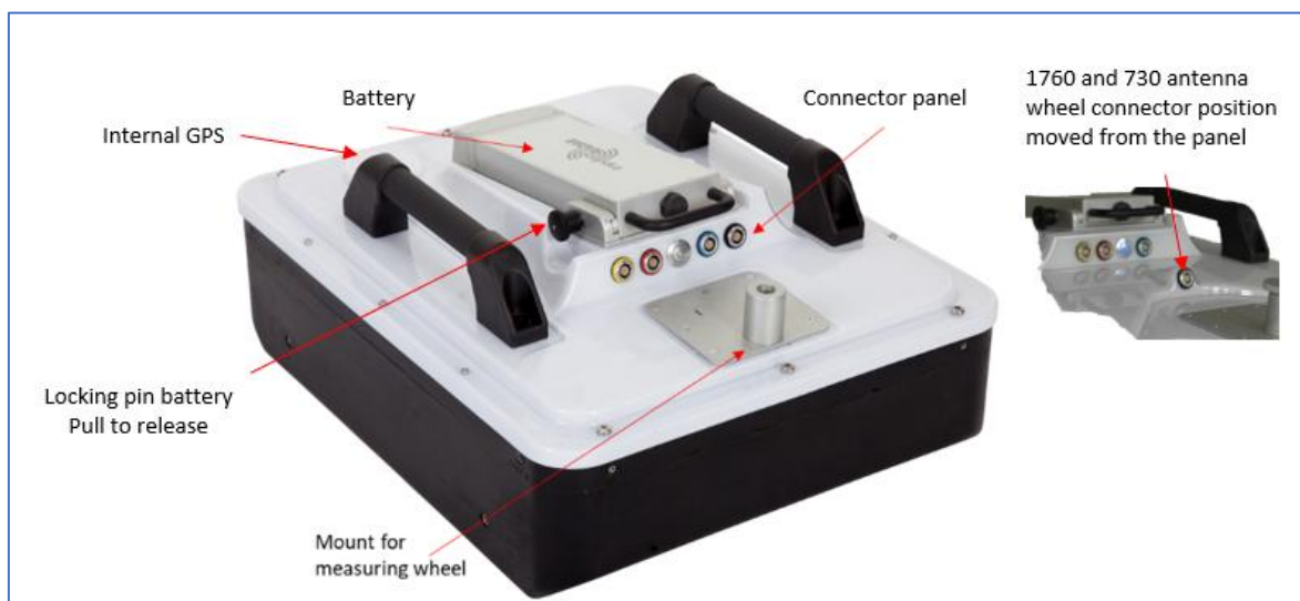
Figure 2 CrossOver 4080 GPR unit with a battery attached.
