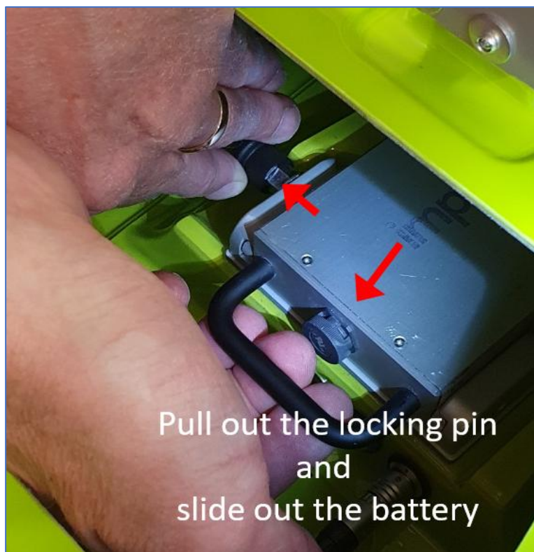
Figure 3 Exchanging PinPointR GPR battery.
