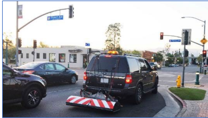
Figure 11 Full survey setup fitted to an SUV
