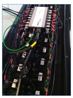
**Note:** ImpulseRadar supply standard carrier solutions in the form of a push-cart and vehicle-mount, which depending on the Raptor antenna type (Raptor-45 [450 MHz] or Raptor-80 [800 MHz]), can accommodate either 8-12 channels or 18-30 channels respectively. Clients requiring bespoke channel arrangements beyond these are responsible for the design and build of their own carrier solutions, albeit with support from us in relation to antenna location, separation, cabling, and power arrangements.
