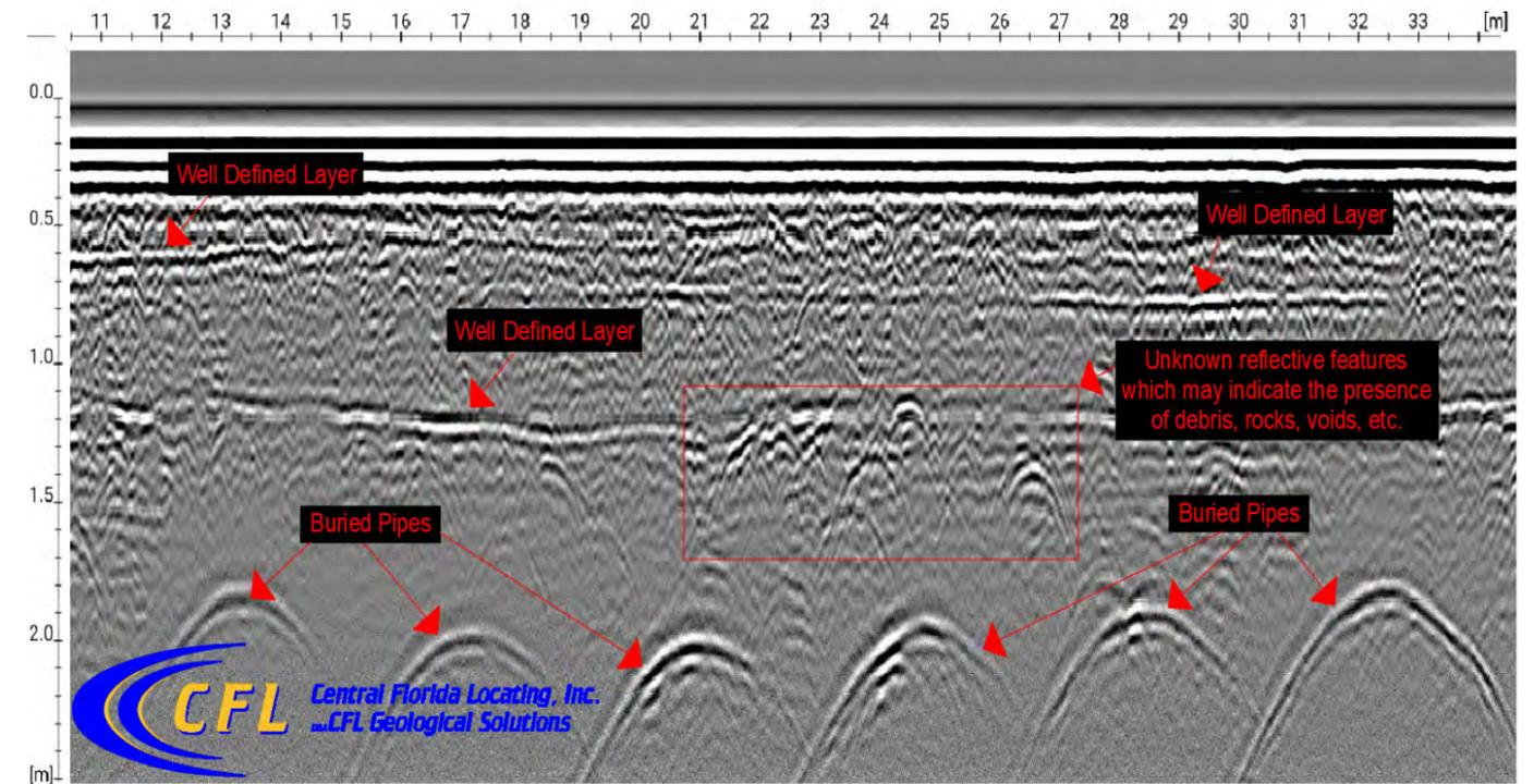
Figure 2: Interpreted 800 MHz data set over culvert bridge system
