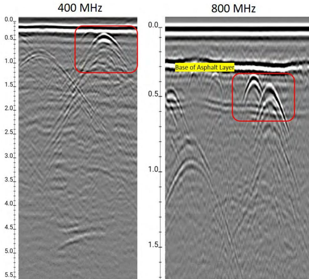
Figure 1: Comparison of depth penetration and resolution over same target area. Vertical depth scale in meters. Useable data to five meters at 400 MHz and up to two meters at 800 MHz. Note target utility couplet not nearly as resolvable at 400 MHz and in the near field/surface.
