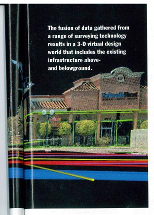
that can accomplish this task," Wolf says. Using a 2-D system would have required lane closures, and each intersection could have taken up to a day to scan, he notes. In addition, the information gathered would not have provided the same density or image quality as this system did, according to Wolf. "The biggest challenge is assimilating all these data into a workflow and
