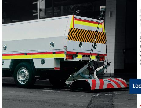
Raptor antennas offer a flexible way to configure multi-channel 3D GPR arrays from as few as 4-channels up to 30-channels as standard, or larger bespoke solutions upon request.
